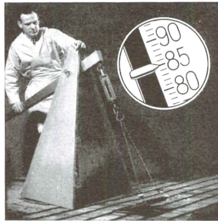
PlyScord holds nails well. Tests on roofs exposed 2 years show minimum force of 85 lbs. required to pull cedar shingle from 5/16" PlyScord. In case of asphalt shingles, roofing is invariably torn from PlyScord without loosening nails. Other tests and actual experience shows 5/16" PlyScord holds nails as well or better than 1" soft pine boards.
