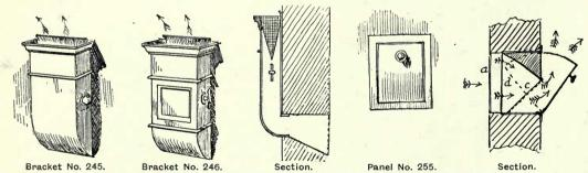
THESE AIR INLETS ARE MADE OF GALVANIZED STEEL AND PAINTED.
