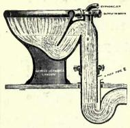
Combines the simplicity of the Cottage Basin and Trap with the advantages of a Valve Closet without the mechanism.
