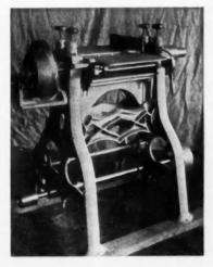
THE cut herewith represents the Planer with the Buzz Attachment on, to dress lumber out of wind, or straighten the edge for glue joints, etc. The rest is made to set at any angle, to use for cutting bevels, or guide the lumber square. The depth of cut is regulated in a moment at at your right hand by a handle moving back and forth. By moving the
