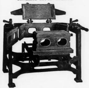
The SUPERIOR makes the stone with the face down or in the bottom of the flask, which permits of the use of fine rich material for the face and coarser, cheaper material for the main body of the block.
