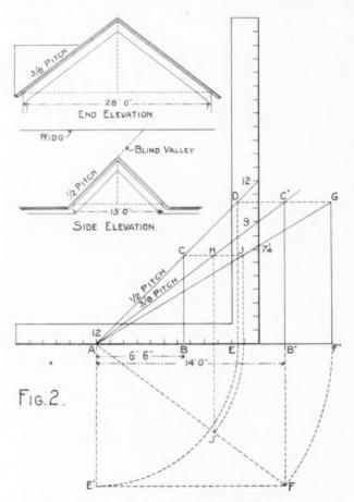
parallel with the one from 17 to 12, and the point of intersection on the blade will be the figures to use for the last application of the steel square to obtain the length for the extra nine and one-half inches in the run. In the case of the half pitch, the rise being equal to the run the figures on the blade are the same as those in the run. This should not be allowed to confuse, as it does not occur in any other pitch. To
