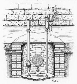
removing waste water from kitchens below the level of the sewer, drippings from ice-boxes and for any purpose where it is necessary to remove water economically from one level to a higher one, the automatic cellar drainer (of which there are several makes on the market) seems to answer the purpose on a small scale very satisfactorily.
