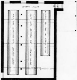
tanks that hold the hard water, and the cistern water required for use on the farm. The tanks are supplied by pumps in the power house and from these tanks pipes are run to the other buildings, water tanks, etc.
