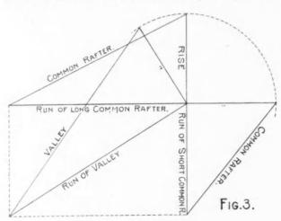
get the length of valley you wish; first lay off the pitches 12 to 12 and 12 to 9 as shown in Fig. 2. Now assuming that the run for the half pitch is six feet six inches and that for the three-eighths pitch is fourteen feet we lay off these lengths
