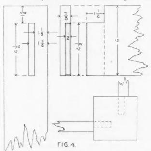
to enter their tenons and mark, measuring first one and one-half inches then four and one-half inches as was just done. These marks locate the ends of the mortises.
