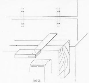
be made of stock which will dress to three-quarters of an inch. In cutting the shelf boards, allowance must be made in the length for the keyed tenons. They should be cut roughly of almost the same length as those of the top. The sum of their widths should approximate two feet in the rough.
