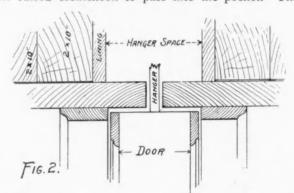
can be avoided by running a stop around both sides of the door and membering with the astragal as shown in Fig. 1. The stop on the jambs are set as shown. Thus, it will be seen that the escutcheon is cleared and that when the door is shoved back, the astragal will cover the pocket opening and to all appearance is simply a mould made fast to the jambs. The head jambs should be set to allow only for the free working of the hanger as shown in Fig. 2.
