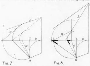
as before, place one leg of the compasses in Z, extending the others to touch the line from m, and turn over to the ground line; a line drawn to o from this point will determine the bevel for the bottom tangent as shown
