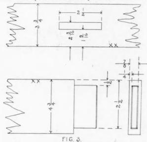
for not planing the boards before gluing them together is because of the impossibility of doweling them so as to make the surfaces match with sufficient accuracy.
