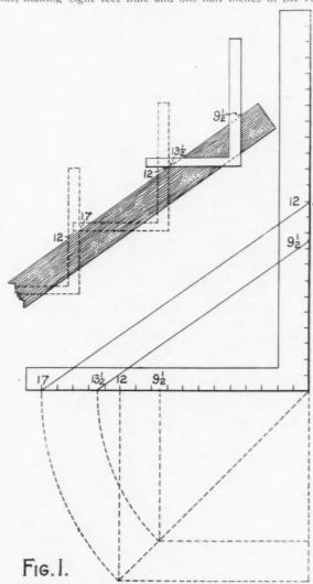
I take 17 and 12 on the square eight times for the eight feet in the run. What I want to know is how to get the nine and one-half inches. Also how to get a valley rafter for a gable of half pitch to fit over another of three-eighths pitch.
