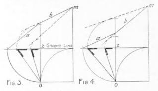
shown in the diagram, is of the same nature as that of the top bevel for a common rafter.
