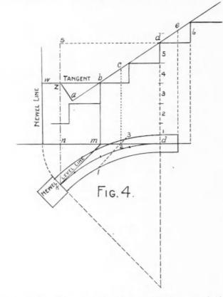
the wall stringer and also on the front stringer which generally in stairways of this class is cut out instead of being grooved.
