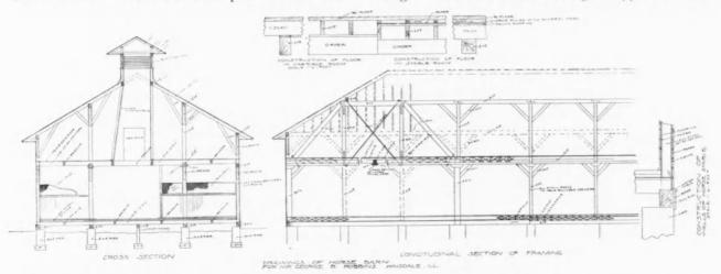
ing plate of the second floor joist. All these timbers are braced at all intersections with 4 by 6-inch braces. The outside walls are formed by filling in between these bents with 2 by 6-inch studding spaced 2 feet pine beaded ceiling, varnished, natural finish.
