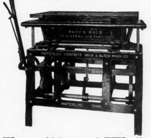
ONE movement of the lever operates the ENTIRE machine, consuming the least time for operation of any machine. Two men will make 250 blocks per day. Our block is patented. Has double, a vertical and horizontal
