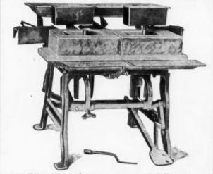
HY not manufacture your own Building Blocks? We have the machine that will do it. The machine that makes the right kind for all buildings. It makes building-blocks from 4 to 32 in. in length, and any height from 4 to 12 in.
