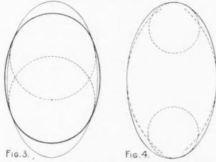
an ellipse. The ends are apparently small circles blending into large circles at the sides, but as it is a continuous blend there is no part of a true circle in an ellipse. The top of the oval and the dotted lines below form a true circle, and it seems to me that this illustration shows three complete and separate figures, an oval, ellipse and a circle.
