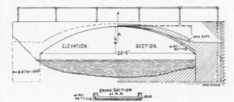
the abutments. By placing the steel and netting within two or three inches of the lower side of the arch the following thicknesses at A, A, will withstand heavy public traffic: Six-foot span, five inches; eight-foot span, six inches; ten-foot span, eight inches; twelve-foot span, nine inches; thirteen-foot span, ten inches; twenty-foot span, twelve inches.
