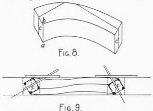
$\alpha$  indicates the length from b equal to the length b w, which is the level tangent shown in Fig. 4. Upon b erect the perpendicular line b k; place one leg of the compasses in b; extend the other to  $\pi v$ ; turn over to k; and connect k b; which will be the level tangent as it is required on the face mold.
