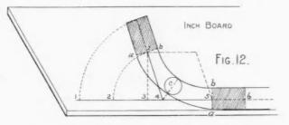
square to the face of plank, and cut the joints also square to the face and square to the tangents. Find the center of each joint as at c and c and place the bevels to cut the centers as shown at c and c in Fig. 9, which illustrates the wreath as it will appear after it is squared ready for the molding.
