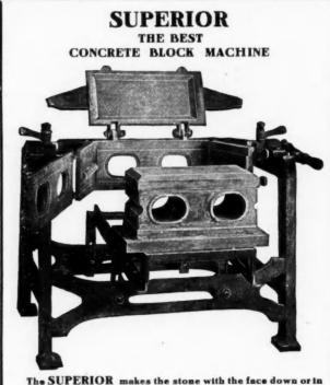
The SUPERIOR makes the stone with the face down or in the bottom of the flask, which permits of the use of fine rich material for the face and coarser, cheaper material for the main body of the block.
