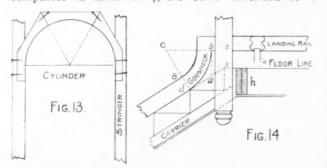
and turned over to 2''. By connecting 2'' to 4 we fix the position of the tangent 2'' 4 as it is required on the face mold; the other tangent being 4, 5. The joints are made square to these tangents, respectively.
