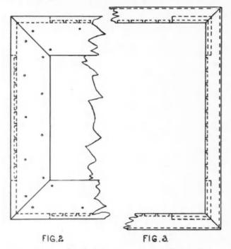
ner pieces are shown in the drawing, Figs. 2 and 3, as mitered; that is, one edge of each is planed to an angle of forty-five degrees to one of its faces. Miter joints are more difficult to make than butt joints. Either kind will answer here though the miter is the one a master workman would use.
