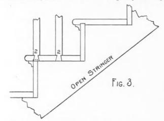
the risers, and 17 on the edge representing the tread. This will help memorizing the number of treads and risers required which in course of construction will be found of some advantage as it will minimize the danger of cutting the stringers too short.
