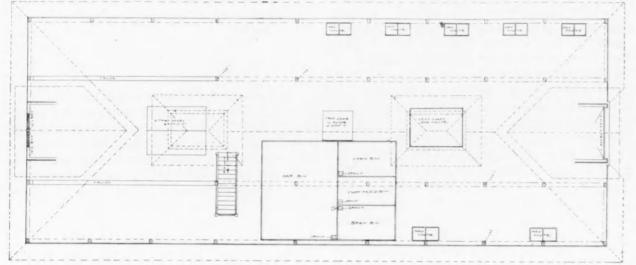
is also covered with paper and then sided with drop at the second-story joist level there is a 6 by 8-inch siding. The roof is of cedar shingles dipped in mosstimber notched in between these posts for the bear-
