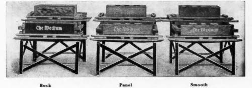
Operates in three sections, mak-ing ROCK, PANEL and SMOOTH face all at the same time. Its capacity is 1,000 blocks per day-ten hours. COSTS ONLY \$200.00. Single sections with all attachments \$125.00. Operates in the MEDIUM PROCESS. Our blocks cost only one-half as much as others.
