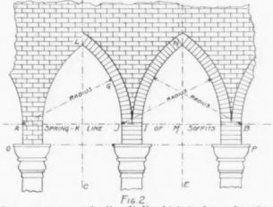
the centres set at the line D-E which is the real spring line of the semicircle, though it cannot be properly termed the actual spring line of the arch itself, and it is at this point we come to what might be termed the "Displacement" of centres. It is usual among mechanics to take it for granted that the centres of the arcs or curves is invariably on the spring line either inside
