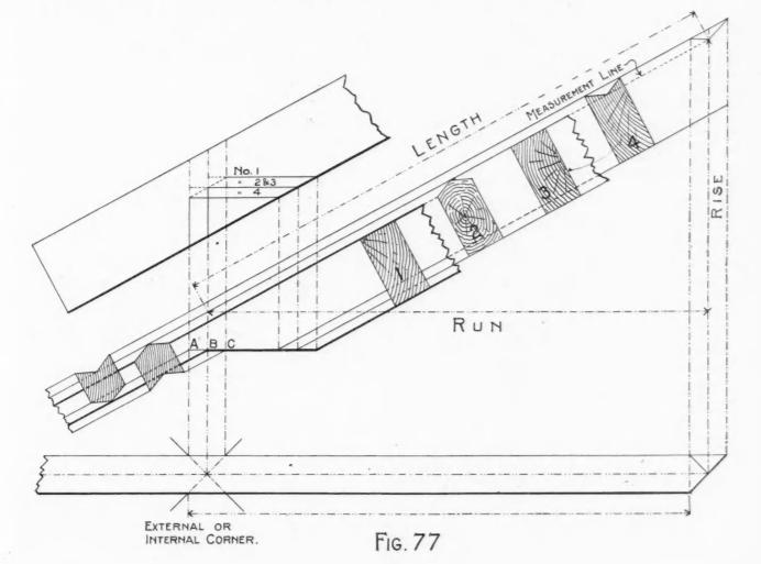
valleys is at a line along the center of the back, and just where to place the square on the side of the rafter so as to make the cuts and length come right at that point is a question that taxes the skill of most carpenters, especially so in the case of the latter, where the same are to be backed.
