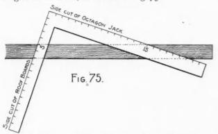
What is true of this, is true of any other polygonal roof. In Fig. 76 we show the tangents on the blade for the polygons from 4 to 10 and represent the figures to use on the tongue of the steel square instead of 12, as in the square-cornered building. In connection with this illustration is shown the figures to use for the octagon as applied in Fig. 75.
