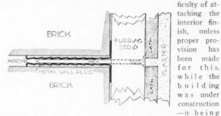
practically impossible to open the joints after the cement has once hardened.
