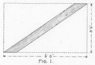
the ordinary brace, but the line of measurement instead of being along the edge of the timber (or a line parallel with it) is on a diagonal line across the face of the timber, as shown in Fig. 2. The run and rise taken to a scale on the
