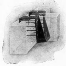
inches long, driven  $3\frac{1}{2}$  inches into the underside of the girders; that is, these headless pins, projecting through the bearings of the post cap, securely anchor the girders and facilitate the falling out of the burned through girders in case of destructive fire without disturbing the walls. The
