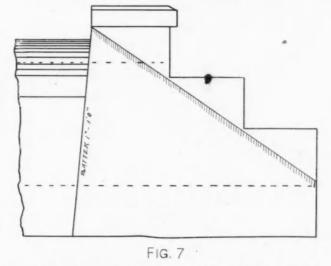
the sides and edge of the board. Or if figures are preferred, we can do as follows: Since we have a 30degree angle and at 90 degrees we would have one inch batter, we find we would have 1/3 of an inch if the wing wall was plumb, but since we have  $\frac{7}{8}$  of an inch batter in the wing wall, we find that it will cut 7/32 out of square and that added to 11/32 will give 9/16 to one batter. This is not absolutely correct, but near enough for all practical purposes.
