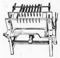
The Reed machines fill the requirements. Blocks and brick are turned out of the mold box under pressure.
