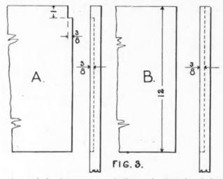
edges of the leg so as to indicate the length of the opening. Set the gauge to three-sixteenths of an inch and gauge on the top and edge of the leg so as to show the depth of the recess. Keep the gauge block against the inside surface of the leg. Be sure the marking is done so as to have the legs pair one with the other. Cut to the lines using chisel and mallet.
