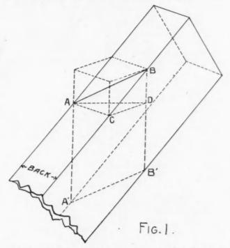
cornered. If it be an octagon roof, then the angle would be at 221/2 degrees. If it be for a hexagon roof, the angle would be at 30 degrees with the sides, etc. EDITOR
