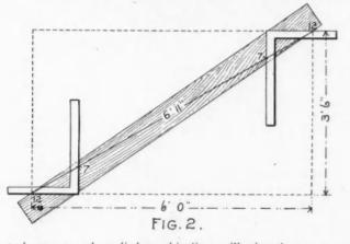
steel square and applied to this line, will give the cuts as shown. The tongue giving the cut for both ends. The figures used on the square can be anything that is in the ratio of those of the run and rise, as 6 and 31/2, 12 and 7, 18 and 101/2. etc. EDITOR.
