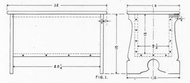
of an inch; or, if desired, both top and under side may be gauged with the pencil gauge to one-quarter of an inch and a round put on the edges and ends as shown in Fig. 1.
