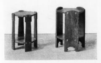
To lay out the sides of the leg, measure from the bottom four and three-quarter inches and square a light pencil line across the face. At the top of the leg square another light line across at the point from which the arc at the top of the leg was described. Set
