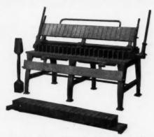
Made in Four Sizes-5, 10, 20 and 40 THE STANDARD CEMENT BRICK MACHINE is the fastest hand brick machine on the market; will make plain, veneered, and ornamental face and shape; all perfect, smooth brick, true to size and design.
