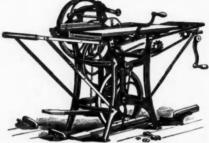
Union " Combination Self-Feed-Rip and Cross-Cut Saw.
