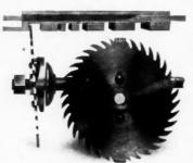
wabble saws. It is provided with side cutters, the kind all wood workers know is best for gaining or cleaning the sides of a groove.
