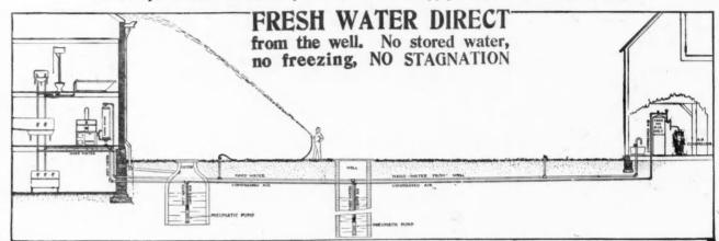
The PERRY PNEUMATIC WATER SYSTEM furnishes water at any given pressure at the faucets by means of compressed air. Power and air compressor operate only occasionally to keep air reservoir charged. This stored air is used, and the Perry Pneumatic Pump operates only when water is drawn. Air may be piped to pumps in widely separated wells. Well and cistern water may be obtained with one air reservoir, as illustration shows.
