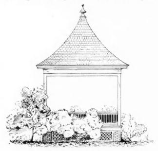
weather surface each time until it is six or seven inches at the peak. The gradually increasing spacing apparently adds to the curve of the roof; and this gives the roof an interesting appearance.
