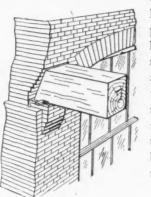
Floor Timber Resting on Cast-iron Wall-plates, With Lugs for Anchoring Timber to the Wall.
