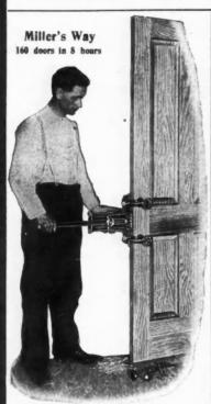
Will cut an opening in three minutes for a mortise lock in hard, soft, crossgrained or end wood, parallel with sides of door.
