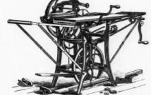
"Union" Combination Self-Feed-Rip and Cross-Cut Saw
