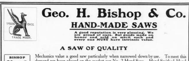
**No.2** Mechanics value a good saw particularly when narrowed down by use. To meet this demand we have placed on the market our No. 2 Hand Saw. Hand Smithed, Hand Blocked, Hand Filed and Set. The life of this Saw is fully equal to the regulation width. The Blade is narrow and shapely. The 26-inch is  $1\frac{1}{2}$  inches at point, and about 6 inches at heel. Shorter lengths than 26-inch, while the same width at point, vary to 5 inches
