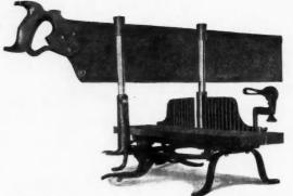
The second cut shows the saw raised to full height so the operator may use both hands in placing stock to be cut. When ready to use the saw all that is necessary is to take hold of the handle of the saw or give the saw guides a light tap on the top and the saw will drop into position ready for use.
