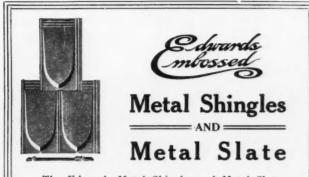
The Edwards Metal Shingles and Metal Slate are made of the best quality Worcester Grade Terne Plate, furnished either painted or galvanized (galvanized after being formed). They can be applied without soldering, the use of special tools and by an ordinary mechanic. A surpassingly beautiful roof covering of extreme lightness and durability.
