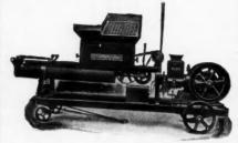
through a perforated pipe, the quantity being regulated by a valve. There are twenty-eight rapidly revolving p a d d l e s which throw the material over and over, thus mixing it more thoroughly and uni-
