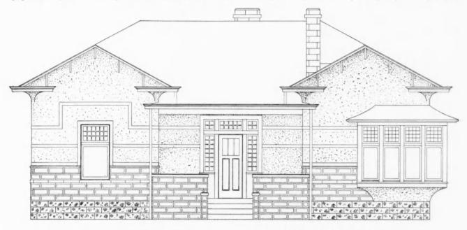
roof is stained a dark green shade and the sash are painted white. The terraced porch is built of the paneled blocks and is plastered on the inside. It is spanned by a six by eight timber which supports the porch roof. The three double-hung bedroom windows reach the four-inch sill course, and the other windows except the oriel and front casement windows, reach only to the water-table.
