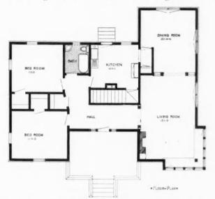
casement windows located three feet three inches from the floor. The large oriel window in the living room provides a roomy window seat; and the upper sash, which are of plain leaded glass and controlled by transom lifts, will afford plenty of ventilation.
