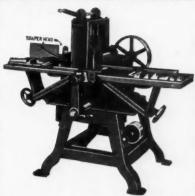
Universal Wood Worker, equipped with our Planing Attachment, will plane up to 4 in. thick and i0 in. wide; also ar-ranged for doing two side molding, match-ing and sticking.
