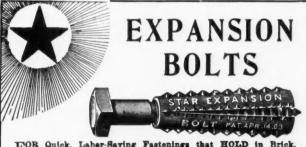
FOR Quick, Laber-Saving Fastenings that HOLD in Brick, Stone and Masonry. Drill hole, place STAR SHIELD within, then put lag screw thro' material to be attached and inte STAE SHIELDS and fasten tight. A positive inside lateral expansion insures a fastening PERMANENTLY DEPENDABLE. Catalog, Samples and Prices upon request.
