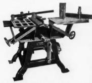
Universal Wood Worker, fitted out with the Single End Tenoning Attachment, with traveling table and hold down lever.
