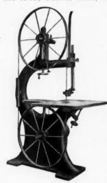
improved 36-inch high-speed band saw which is giving such universal satisfaction wherever installed. The frame of this machine is a very heavy cored casting with ample floor space. The wheels are built up, that is the hub is bell-shaped to allow the bearings to extend beyond the center of the wheel. The spokes are of solid steel and the rims of the wheels are of steel, electrically welded, and then ground perfectly true and covered with an endless rubber band.
