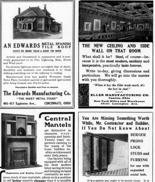
It is a system you ought to be posted about. It is both simple and effective. One man can hang the lath on the prongs and clinch them securely with the tap of a hammer. Berger Prong Locks save time and money. There's no wiring and the lath can't get away.
