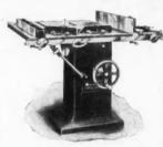
This machine is a dandy. It is strongly built. The arbor moves up and down in an arc so that the belt is always tight. Equipped with four gauges, two saws and counter shaft, including our splendid gear operated double acting, tilting, ripping fence.
