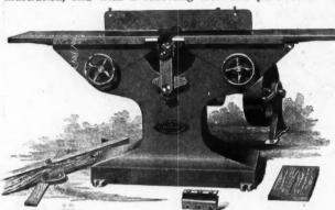
will take a cutter-head up to 9 inches long, one of this size being furnished with the machine, same being either the company's patent triangular shear knife head or a slotted head as may be preferred. Other heads for any required purpose are furnished upon order.
