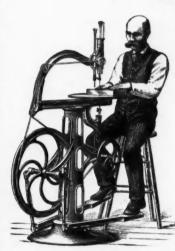
Suitable for carpenters, pattern and cabinet-makers and all wood-workers requiring accurate work, also for sawing soft Will cut up to 3 inches thick, swings 24 inches, has powerful tread motion, cuts rapidly and is easy to operate. Has adjustable tension spring on upper spindle, dust blower, drill attachment, iron tilting-table, etc. Will furnish tight and loose pulleys for power in place of treadles when desired.
