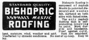
Bishopric Roofing is composed of Asphalt Mastic (a patented discovery) and woolen felt, surfaced on both sides with flaked mica.
