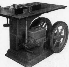
The All-Iron Rig, as shown here, weighs 1150 pounds, crated—the Engine being a strong six-horse, and pulls 14-inch saws
