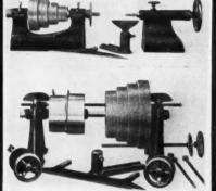
Wood Turning Lathe and Countershaft
