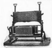
"The Miles" No. 5, Down Face, Wet Concrete Block
