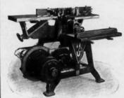
Individually driven Machines can be placed where they are most convenient as regards light and easy handling of material, entirely independent of the shafting.
