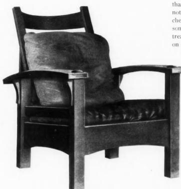
the bevel square will be needed in marking the shoulders. The arms are to be bent; a curved form slightly more curved than the arm is to be, will need to be prepared upon which to clamp the arms after they have been steamed. Curved forms will be needed for the back horizontals, too.
