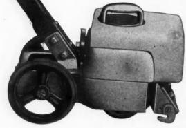
This extra weight adds 40 pounds pressure over the cutting edge of blade and will force the knife into the hardest wood surface. As this additional weight is only required while scraping old floors or some special grades of new hard wood floors, it is so constructed that it can be attached or removed in a few seconds time.
