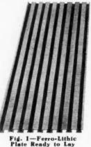
demand for a permanent, fireproof concrete roof. The application of these plates has been extended into other fields and they are now extensively used for centering and reinforcing
