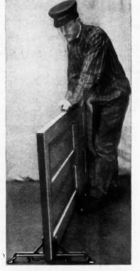
the clamping faces are padded to prevent injury to the work. The clamp may or may not be fastened to the floor.
