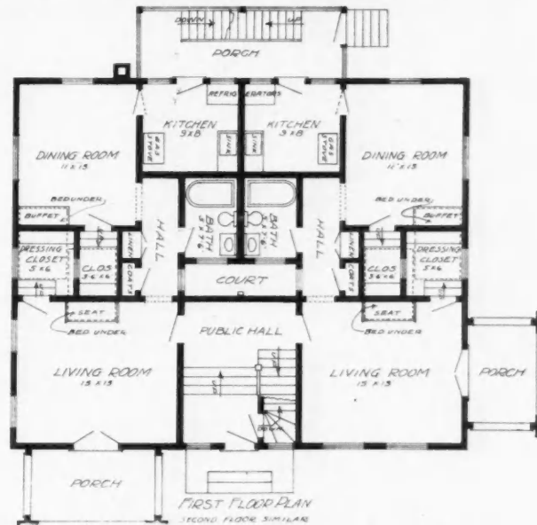
3-Room Apartments with Accommodations Equal to 5 Rooms
