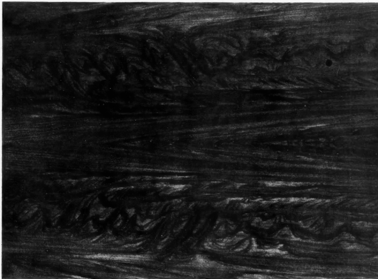
Panel of Richly Marked Red Gum Veneer (About One Quarter Full Size)
