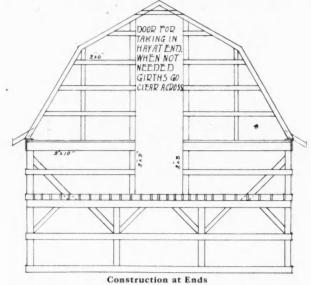
the plan was first presented and not one has given trouble to erect or in use, so far as I have learned. Siding on this barn is better put on vertically. If matched siding is desired it works as well vertically as horizontally. The building may, however, be studded and siding put on horizontally. In building the joist frame barn the following directions may be of value:
