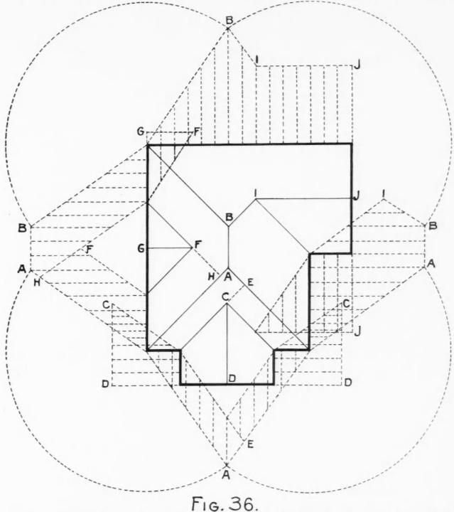
Now, we will show the same formula applied to a hip roof with gables as shown in Fig. 36. In this are this method, aside from laying out a true diagram but shown all of the rafters for the different sides. When set in place in the roof-that is if we could fold over these sides directly above the plan-like letters will come together and show as but one letter at the inter-
