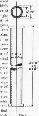
equals  $10'' \times 10'' \times .7854$  or 78.54 square inches. The area of a 8-inch circle equals  $8'' \times 8'' \times .7854$  or 50.26 square inches. Subtracting 50.26 square inches from 78.54 square inches, we get a memainder of 28.28 square inches, which is the area of the cross section
