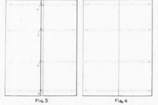
accurately bored, and there should be more than two of them. If the boards are carefully selected as to grain, and the rods are spaced not more than four or five inches apart, the completed job will be as secure as if cleated. W. D. GRAVES.
