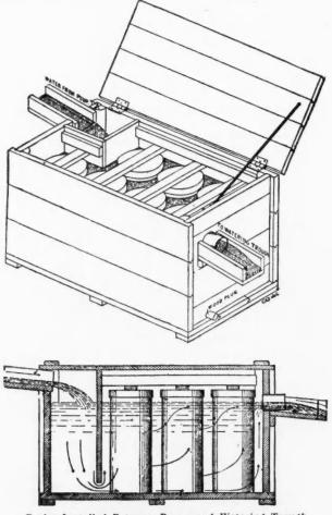
Cooler Installed Between Pump and Watering Trough
