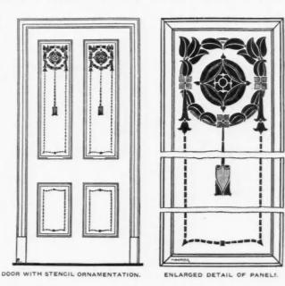
terial, such as paper or zinc—the stencil—a pigment is brushed over the plate with short, stiff brushes made expressly for this purpose, and the color passing through the stencil plate on the surface of the work leaves an impression.
