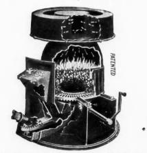
Underfeed Boiler, Cut Out to Show How Fire Burns on Top
