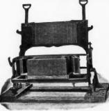
"The Miles" No. 5, Down Face, Wet Concrete Block Machine
