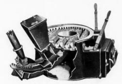
The Boiler Underfeed Device
