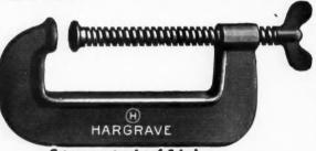
This clamp is thoroughly made of the best refined malleable iron, and is provided with a button tip. It has a very deep, square thread in both the screw and frame, and is in every way the strongest and best clamp in the market. Each size is numbered by inches the thickness of the work it will take in.
