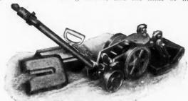
power necessarily confines the operator of a "dead weight" to a small, light machine with a correspondingly small capacity. In the "Spring-Driven" floor smoother, where the effort is equalized between the push and the pull a larger and more effective machine can be used, which naturally will not jump and leave waves, and at the same time enables the operators to do twice the work with half the effort.
