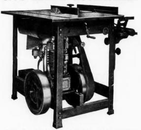
TYPE A with 4 H. P. Gasoline Engine. Weight 400 lbs. Showing only Rip Saw and Jointer. 7 Other Attachments
