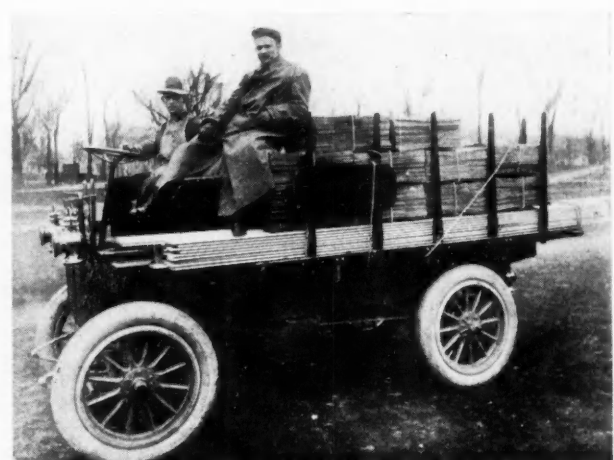
Ferry Lumber Co., Pittsfield, Mass., Making Good Use of a 1,000 Pound "Franklin" Gasoline, Air Cooled Truck
