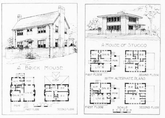
windows opening from the living room. Direct communication is also had from the kitchen to this porch. The combined front and rear stairway form a good feature of this design. The second floor contains large, well lighted bed rooms with ample closets and a convenient bath room.
