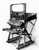
a blow absolutely parallel to the bottom of the mold; thus the result is a uniformly tamped product, and one densely compressed. The impact of this tamper with the material is so intense that only two blows are necessary to produce a set of ten bricks. Note the speed that this would permit.
