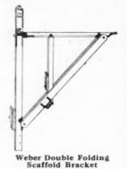
Without loosening a single bolt, it can be quickly folded into a piece so small that 12 of them will not take up any more room than the ordinary tool chest. This feature will appeal to every contractor, as it greatly lessens the haul to and from jobs, and saves the time of the workmen.
