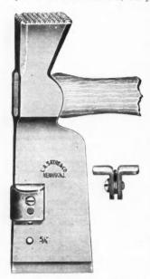
an outgrowth of the loose gauges that have been in use on the Pacific Coast for a number of years. The loose gauges, however, have never met the requirements in shingling as they would shift on the hatchet, thus changing the lap of the shingle.
