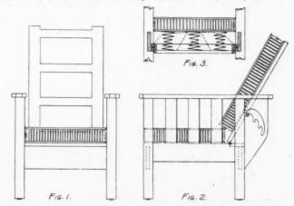
and the simplicity of construction. The legs are 22 inches apart in each direction, which gives ample room between the handles, and simplifies the work on the end and side rails, as shown in Fig. 5 and rail marked "C" just below the figure. The adjusting brackets F in Fig. 5 are so designed that they occupy the minimum space and permit the cross bar, supporting the back, to be the same distance from the hinges in its different positions. The pocket in the brackets F, Fig. 5 are
