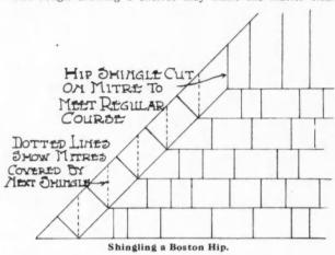
In laying the best practice is to stop regular courses when tip of shingles in each course reaches ridge of hip. Then snap lines each side after rest of roof is completed; and these snap lines will serve to guide straight edge used in marking new shingles laid to complete the courses.
