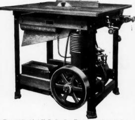
Type "A" with 4 H. P. Gasoline Engine, showing Rip Saw. Weight equipped for work 350 lbs.
