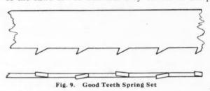
ened by one stroke of the file, they should be gone over the second time before the file is advanced in the clamp as this will save one half the time of changing the saw which is considerable.
