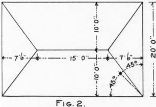
would be at 45 degrees with the cornice line; but what would the run of the hip be for the same roof with a ridge 15 feet long and could I find the side cut of the jack as shown, by the diagram in the May number?
