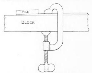
Fig. 3. Block of Wood Clamped to End of Broken Saw
