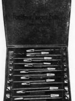
Guided by its circular rim—instead of its centre—the Forstner Labor-Saving Auger Bit will bore any arc of a circle, and can be guided in any direction.
