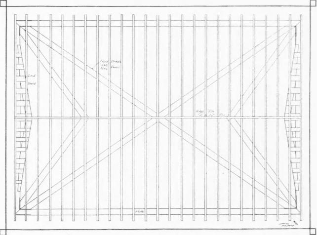
Roof Plan, Showing System of Bracing
