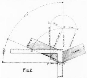
the part covered by the square, as bounded by ABC forms a triangle which will represent the plan; and by the addition of the desired rise, the length and cuts of the rafters may be determined, as shown in Fig. 2. Here is the same angle of corner, as shown in Fig. 1, to which is added the developing lines, as follows:
