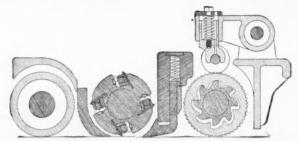
Diagram Showing Relative Position of the Feed Rolls, Cutter Head, Chip Breaker and Pressure Bar, and Incidentally Showing Construction of New Round Head, Patent Sectional Chip Breakers and Method of Giving Pressure to Patent Sectional Feed Rolls
