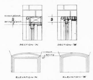
Diagram Showing Parts in Segment Head Windows
