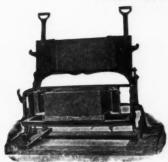
3-Hoppers, Continuous feet Rolling Mix, Low down Steet frame. Simple Strong and Accurate.
