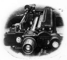
Top View of Cabinet Planer, Showing Grinding Attachment and Implement for Holding Head while Grinding the Knives to the Proper Cutting Angle After Being Jointed
