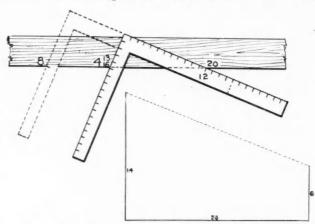
the difference between the two sides on the tongue, and the span on the blade; mark both sides. Then slide the square down to the figure 12, keeping the blade to the lines; and the figure on the tongue gives the number of inches rise per foot run. Having found these proportions, then step off in the usual way.
