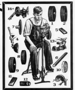
14 Machines in one, including wheels and attachments for all shop grinding, gumming saws, sharpening chisels, plane bits, etc.
