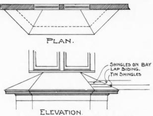
Octaogn Bay. Roof Should Not Run Clear to Sill
