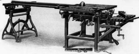
Our table extension is framed together, trussed to prevent springing and provided with steel lumber roll, at outer end. in place it is solidly secured to main table. It can be easily put
