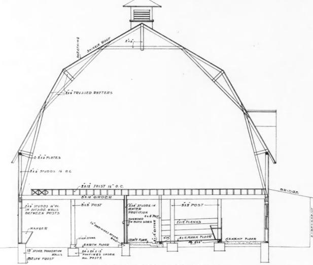
Cross Section Showing Self Supporting Roof Framing
