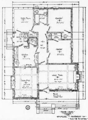
Plan of Concrete Bungalow of W. H. Riley, Riverside, Cal., Built under the Van Guilder System of Hollow-Wall Construction
