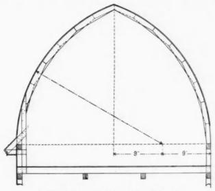
Gothic Roof Curve Built up of 1-inch Plank
