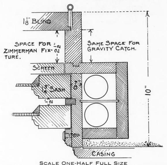
Detail No. 14. Outside Blinds for 10 Inch Wall.—Note that there must be a space of at least 2½ inches between Screen and Blind for Zimmerman or Gravity Fixtures
