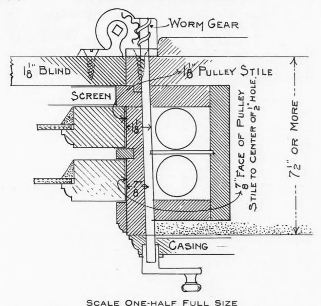
Detail No. 15. Outside Blinds for 7½" to 8" Walls, Showing Arrangement for Mallory Shutter Worker
