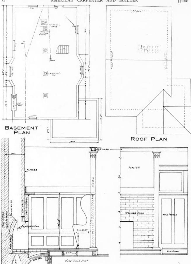
CROSS SECTION AND ELEVATION THROUGH INGLE NOOK AND FIRE PLACE
