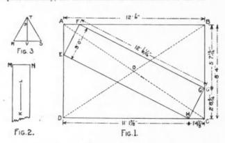
First (in Fig. 1) I located the center of the rectangle A-B-C-D, by drawing the diagonals A-C and B-D and O the point of their intersection being the center. This point would also be the center of any other rectangle inscribed within A-B-C-D.
