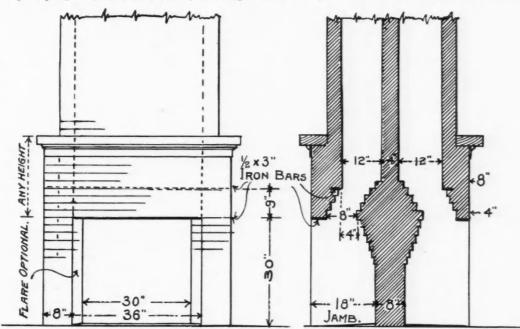
FRONT ELEVATION OF WOOD BURNING FIRE PLACE.
