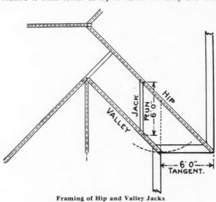
must be a reduction in the length of the jack which amounts to the diagonal thickness of either hip or valley (provided they are of like thickness) and this amount should be set off square back from the plumb line found for the full run. To find the cut across the back, take the tangent and the length of the jack for the full run and the side of the square that represents the length will give the angle for the cut.
