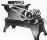
Is used for Jointing, Planing, Moulding, Beveling, Rabbeting, Grooving, and any other work that any Jointer can be used for. We furnish it with or whithout a countershaft, bench or motor. Just as you desire. The Best machine for the money on the market. We make 6 larger sizes, and Wood Lathes, Shapers, Planers, Cut-off Saws, Band Saws and Saw Tables.
