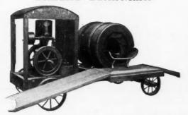
"The Standard" is low charging. The materials are charged into the mixer from platform about two feet from the ground, avoiding building high platforms with long runways or purchasing complicated charging hoists and hopper arrangements.
