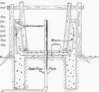
Cross-Section Showing Forms and Tank with Reinforcement
