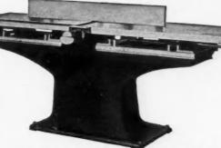
Used for Planing, Jointing, Shaping, Matching, Rabbeting, Grooving, Chamfering, Beading and Making Mouldings
