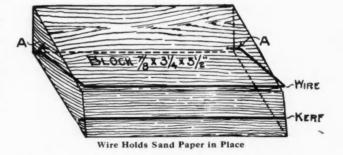
Make two small holes at "A," "A" and bend a piece of wire to the shape and size to just fit snugly into the holes and come down onto the beveled edge. Insert the paper in the kerf, hold with two fingers and bend down under and on around the block until you can clamp it fast with the wire.
