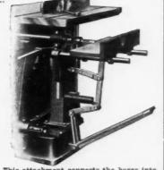
This attachment converts the borer into a hollow chisel mortiser, suitable for cutting mortises up to 5% inch square.
