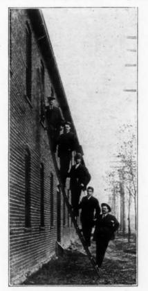
Light Weight, Wire Trussed Ladder in Severe Test
