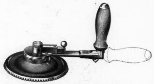
Fig. 3. Showing the Two Positions of Handle
