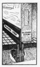
End View of "Schoulers" Patent Weather Tight Door Sill
