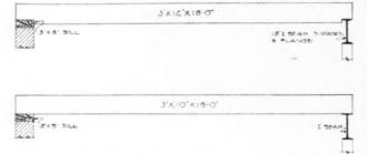
3x12, Cut Down 21" at ends is stronger than 3x10
