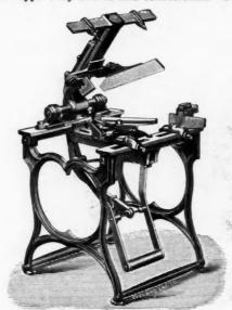
Machine for Trimming and Punching Slate
