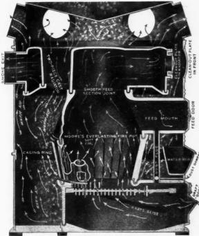
It is a proven fact that MOORE'S FUR-NACE is so constructed that it saves fuel and keeps the house warm in any weather. You get more heat per pound of coal out of MOORE'S FURNACE than from any other make. The reason for more heat is
