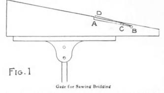
lengths and bevels as are most apt to be required for bridging between floor joists. He thus not only saved quite a bit of lumber but made quite a saving in the cost of cutting. His machine hasn't a swinging cutoff gage, so he got the desired bevel by screwing a wedge-shaped block to the front of the square one he has.
