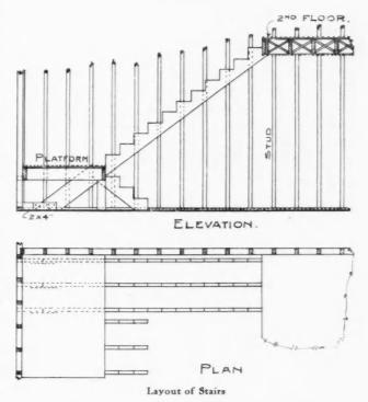
floor,-the rough platform, to the studs under rough horses and to the second floor header; this was to help stiffen the stair and help hold up the center of the joist on second floor. I think this a good stunt; here is an illustration.
