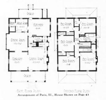
hardwood floors; the remainder of first floor is a large kitchen with work room and pantry attached, built in cabinets and closets, and a large rear porch wainscoted and inclosed with storm sash and door in winter and screen sash and door in summer, a lavatory and closet complete this floor.
