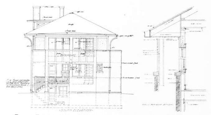
REAR ELEVATION AND MAIN ROOF AND WALL SECTION
