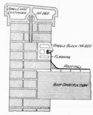
SECTION THROUGH TIRTEEN INCH COPING BOTH SIDES CLOSED
