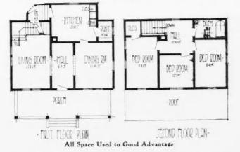
a slapdash finish. Cellar floors are concrete. The building is balloon frame, sheathed with hemlock. Studding 2 by 4, floor timber 2 by 8, ceiling beams 2 by 4, rafters 2 by 4 covered with N. C. sheathing, black Neponset paper and Edwards Spanish metal tile. Outside is covered with galvanized metal lath and stucco, finish same as number two sandpaper, with white Atlas cement.
