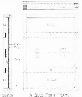
assembled, care being taken to leave the frame square and out of wind.
