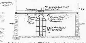
Method Advocated by the Old Builder to Prevent Reverse Currents in the Cold Air Box, also a Re-circulation Inlet for Use During Dust or Sand Storms, and the Furnace set so as to Favor the Registers on the Windy Side
