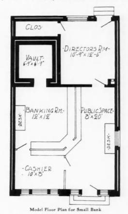
which are desirable in such a building are provided here. It will be noticed that the vault is built with a very thick double brick wall with dead air space between. The ceiling and floor of the vault should be of similar construction and the vault should rest on an independent foundation carried down to a solid bearing. It is important that a bank vault should be built fire-proof. All of the rest of the building may burn and tumble down; but the vault should be made so it will stand. EDITOR.
