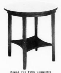
the facings. The steamed parts will have a slight tendency to straighten when released. Another way would be to saw out backings upon the band saw to the radius required and then veneer these with the quarter sawed oak.
