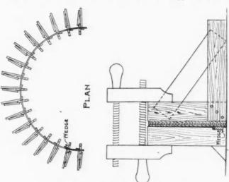
Method of Gluing and Clamping Circle Soffit
