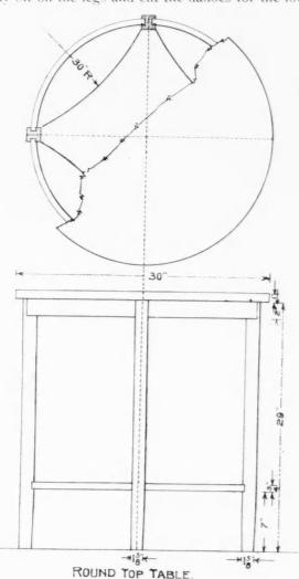
shelf and also lay off and work the joints at the tops of the legs into which the dovetails of the facings are to be fitted.
