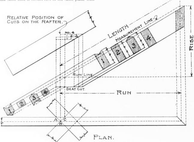
Explaining the Measurements and Cuts of Hip Rafters
