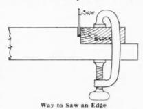
against, the saw would run off, thereby making a ragged cut. He then clamped a block against the joint and cut between the block and the piece and the trick was done.
