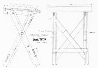
Working Drawing of Collapsible Drawing Table
