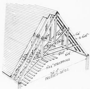
Fig. 1. Truss Construction for Curved Ceiling Church Roof
