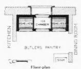
This refrigerator is 6 feet 6 inches wide by 2 feet 2 inches deep by 4 feet 5 inches high. It is lined with opal-glass and the exterior is finished in white enamel to match the surrounding woodwork.
