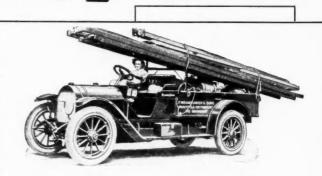
Nickel or Chrome Vanadium steel—heat-treated—fortifies each vital point in a Kissel-Kar truck chassis. Axles both of the heaviest forgings. Cone leather-faced clutch. Spicer Universal joints. Driver's comforts. Bodies built to suit.
