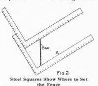
edge, A, of one of the squares will give the angle at which a gage, or fence, must be set in order to do the work. Fasten this gage, which may be any straightedged piece of board, back from
