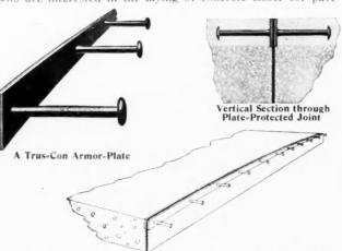
Trus-Con Armor-Plate for Protection of Expansion Joints in Concrete Pavements. Curve adapted to crown of road. Asphaltum felt, \( \frac{1}{4} \) in., between plates, cuts entire depth of pavement
