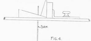
Jig for Working Drip Mould
