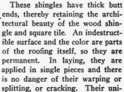
formity of size prevents waste in laying and reduces the cost of application. By using Rex valley strip, the expense of metal valleys and ridges is done away with. Beginning at the eaves, the first course is laid double in the usual manner, always nailing through the under-bent over-end. This fastens the butt of the shingle as well as the upper portion. See The other illustrations show the method of
