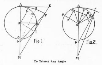
of intersection (H and K) are always equidistant from the point A, if the distances are measured along the arcs, and not as cords between these points.
