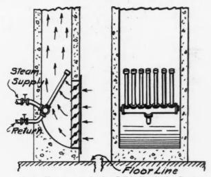
Steam Heater or Aspirating Coil in Ventilating Duct
