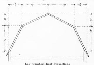
give the upper pitch. For illustration, for a building 30 feet wide, the proportions would be 5 and 10 and 10 and 5 respectively.
