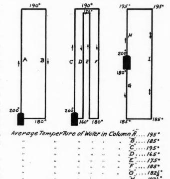
Fig. 1. Diagrams Illustrating Principles of Hot Water Circulatio
