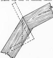
allows nailing at top and bottom of joint. The cut on lower rafter is easily obtained by making a plumb mark (see dotted line) and using the figures for pitch of the roof from that
