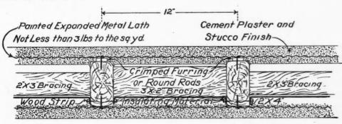
Detail Showing Section of Exterior Wall "A" Type of Stucco Wall
