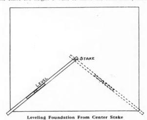
level with straight edge in every direction to where I want my walls, and drive stakes so that the top of foundation stakes are level with center stake. If foundation is a large one, I use two or more center stakes. I find this a more correct way than to start at one corner and level around building, as a great many do.
