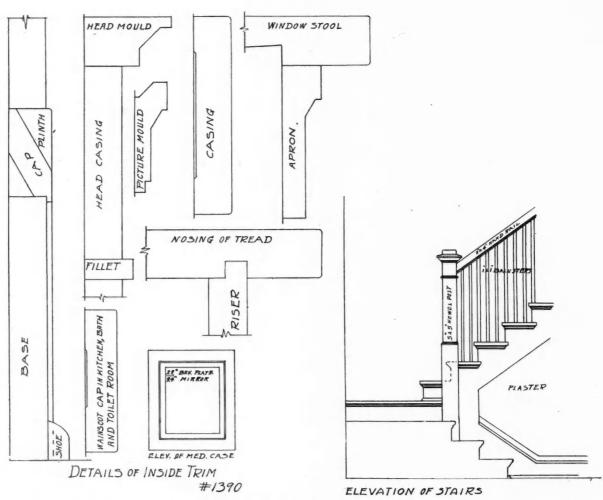
FRONT ELEVATION, SECTION AND INTERIOR FINISH DETAILS OF COTTAGE SHOWN ON PAGE 73
