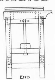
Adjustable Wooden Sanding Table Used in Connection with an Old Turning Lathe
