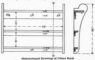
in the other two shelves should be about 134 inches from the back edge. If you cannot get them grooved at the mill and have no plow to do it yourself by hand, then nail very small strips on the shelf as shown in the small figures.
