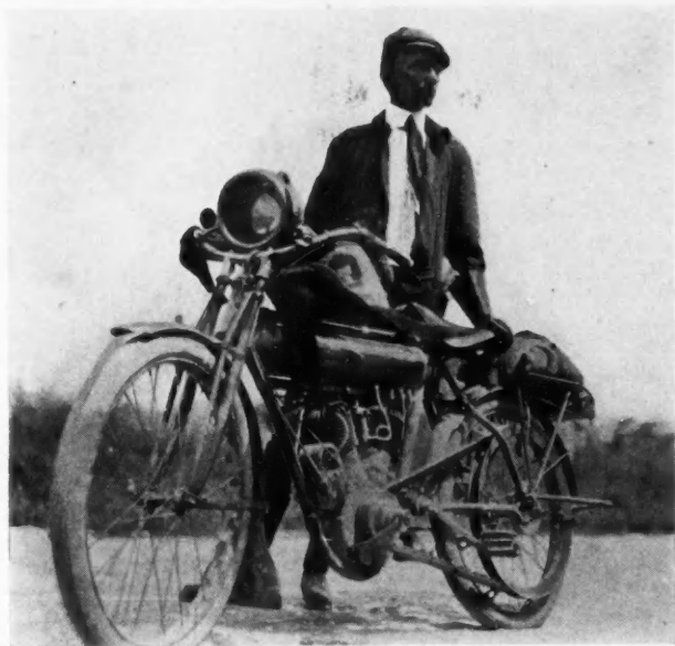
Mr. Ferd Karl, of Canal Dover, Ohio, and his Flying Merkel Motorcycle Have Made a Most Remarkable Record for Economy. He Purchased This Machine, Which is a 6 H. P. Twin Cylinder Belt Drive Model, in 1911. Since That Time the Only Expense Incurred for Mechanical Parts has Been $1.50 for two New Inlet Valves. M. Karl has Covered 39,864 Miles to Date.
