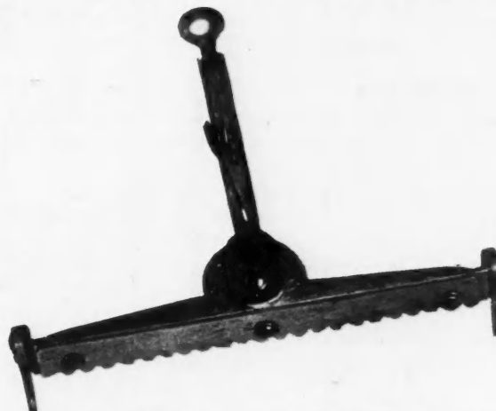
Adjustable Gage and Marker for Corner Board Marking
