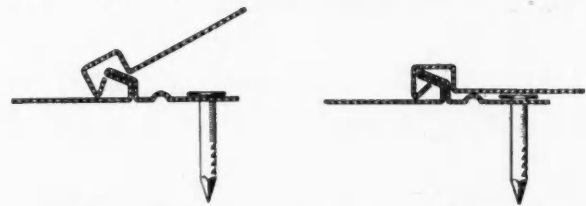
Position of Shingles When Laying or Locking Together. Showing the Shingles Laid on the Roof and Locked.
