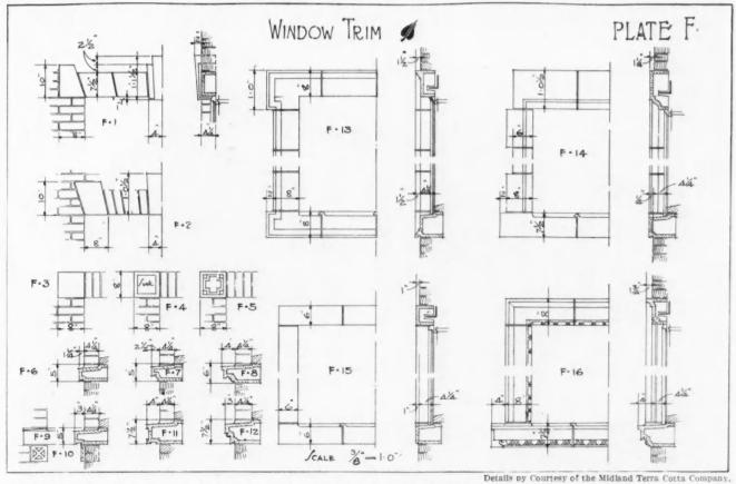
Suggestive Details for Windows Made Attractive by Use of Stock Terra Cotta. In this Plate Simple Terra Cotta Forms Are Combined in Different Ways to Produce Nine Separate and Distinct Designs of Window Trim; Scale & Inch Equals One Foot.
