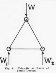
connection with the truss diagrams.
