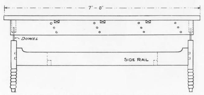
Side Elevation of Collapsible Work Bench. This One was Made Out of An Old Bedstead. Any Stout Frame Work Would Do as Well.
