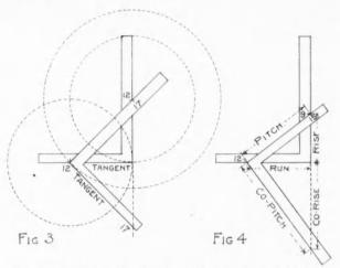
The Angles Formed by the Aid of the Steel Square for the plan and Pitches.
