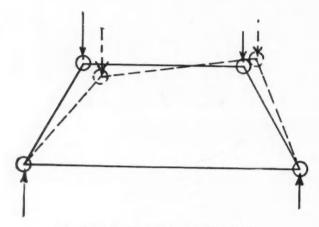
Fig. 10. An Easily Distorted Framework.
