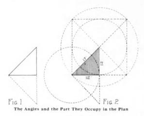
a problem based on the divisions of the circle from which the angle emanates. Therefore, the framing of a roof has its beginning in the circle. It takes on the form of polygons. The equilateral triangle being the first, contains within itself the proportions to form all other polygons and all other angles required in the framing of the roof. In short, it is the beginning and the end; it takes on the beginning as it takes on its first shape and the end where it ceases to have shape.
