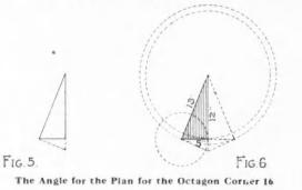
corner, as shown by the shaded part, regardless of the size of the roof and represents the full scale to one foot run of the common rafter.
