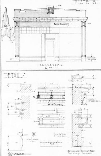
Front Elevation of Pretty Little One-Story Store Buildings to be Built of Brick, Enameled Terra Cotta, and Plate Glass. Below are Details Drawn to # inch Scale Showing Proper Construction for This Building and also for a Two-Story Building of Similar Design.
