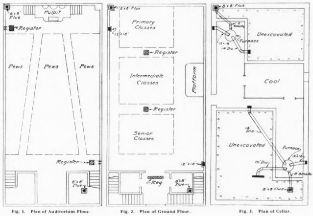
me and I arranged it so that the church had the full use of the Sunday-school floor with no objectionable pipes exposed and with a very small additional expense for excavating. In fact, the entire cellar required did not amount to 40 per cent of the area covered by the building.
