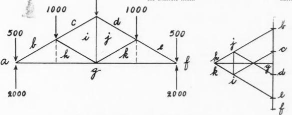
Fig. 12. Stress Diagram for King Post Truss.
