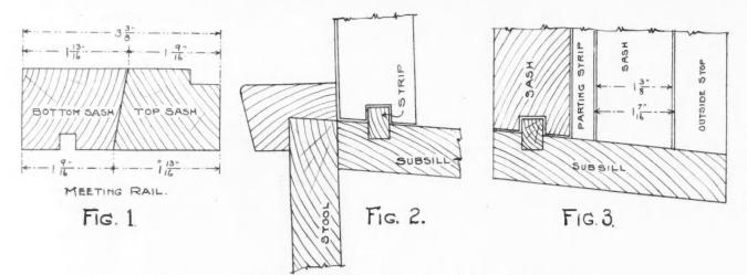
Details of Window Framing Offered As an Improvement Over Ordinary Methods.
