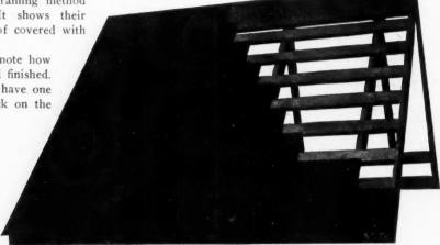
Open Boarding for Slate Roofs Recommended by the Slatington Slate Co.
