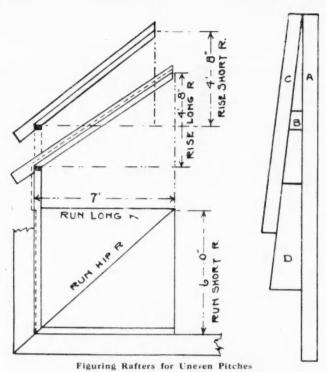
12-inch for seat cut; cut on 9 4/12-inch for plumb cut.
