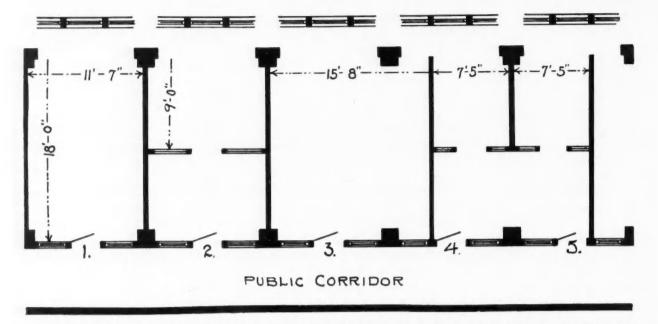
A Typical Office Building Lay-out, With a Public Corridor Along the Inside and the Bank of Offices Eighteen Feet Through to the Outside Windows. (In this Drawing the Windows Are Set Forward Out of Their True Position.)
