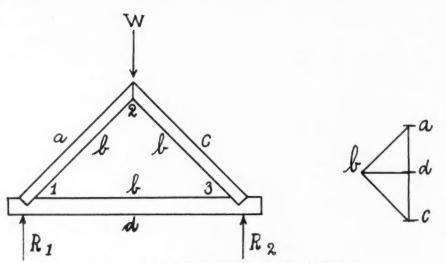
Fig. 11. Graphical Solution Applied to Simple Truss.
