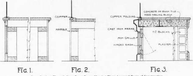
Cross Sections Through Store Front Bases, Showing Three Approved Types of Construction.
