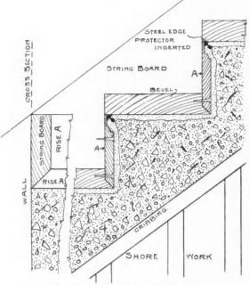
Forms for Making Reinforced Concrete Steps.
