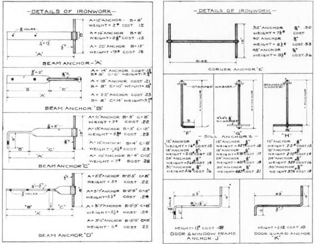
Iron Work Frequently Required in Connection with Brick Construction.
