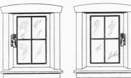
Recessed Casement Windows are Sometimes Trimmed with this Style Fast. These Fasts are Made Handed and Very Often We See the Right Hand Placed on a Left Hand Sash and the Left Hand on a Right Hand Sash.
