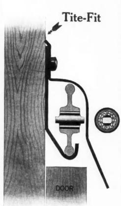
Sectional View Showing Storm Proof Feature, Perfect Tread for Wheels and Roller Bearings with which Wheels are Equipped.
