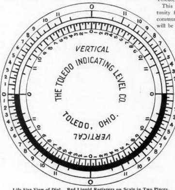
Life Size View of Dial. Red Liquid Registers on Scale in Two Places, Insuring Accuracy.
