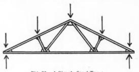
Fig. 22. A Simple Steel Truss.
