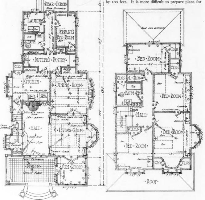
First Floor Plan of Specimen Design.
