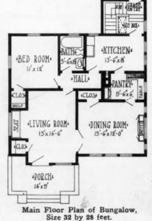
in size, being 5 feet 6 inches by 8 feet. This width gives room enough to turn the bathtub across the far end of the room. The bathroom, besides containing the usual bathroom outfit, has also a medicine cupboard built in the partition. This medicine cupboard has a plate glass mirror fitted as a panel in the door.
