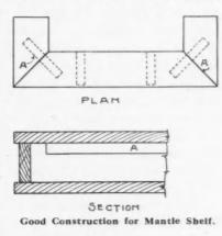
shelf and bottom board, which helps to hold the miter in place.
