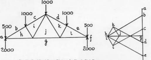
Fig. 23. Dead Load Stress Diagram for Simple Fink Truss.
