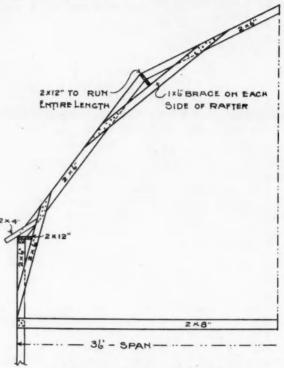
Construction for 36 ft. Span Gambrel Roof.
