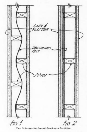
We are showing two common methods that are usually employed to prevent the passage of sound through a frame partition.
