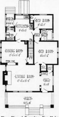
Floor Plan of Bungalow, Size 25 by 40 feet. wide treads. There is so much running up and down stairs from the kitchen to the cellar that special attention is given to this feature. Over the cellar stairs steps to the upper floor are placed. In this house the second floor contains one good room besides storage space.
