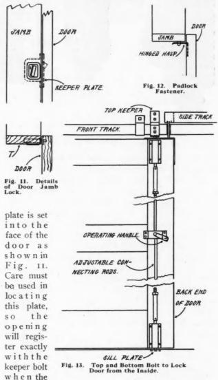
door strikes the stop, R. Notice that this arrangement is just opposite to the customary practice of setting the lock into the door and attaching the keeper to the jamb. The door must lap the jamb at least  $I_{2}^{1/2}$  inches.
