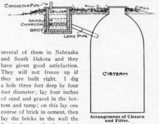
four inches of space between the brick and dirt wall and fill this space with sand and fine gravel. This will keep the brick wall from bursting in at a temperature of 42 degrees below zero, which has been proven. About four to five inches up from the bottom, put in a lead pipe to the cistern; four inch tiling is all right for this purpose. A screen should be put over the filter end. The walls should extend a little above the ground and have a tight cover to keep out insects.
