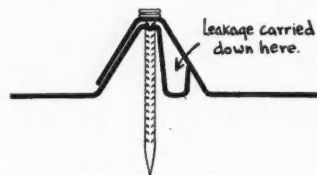
Patent Leak-Proof Joint for Corrugated Sheets.
