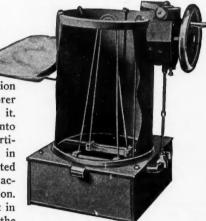
Century Bag Cleaner, Hand-Operated, with Counter Attached, also Bag Shelf; Frame Partly Cut Away to Show Vibrators over which Bag is Dropped.
