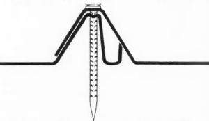
The Patented No-Leak Joint of Moeschl-Edwards Roofing.
