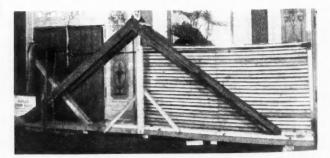
Panel of Stucco Board Construction in Test Frame. This Panel uled at 4,400 Pounds, as Against 800 to 1,400 Pounds for Lath This Pan Failed at and Sheathing Panel.
