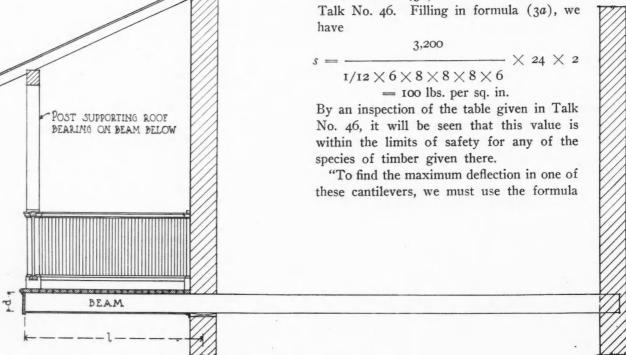
Fig. 4C. Cantilever with a Combination of Uniform Load and Concentrated Load.
