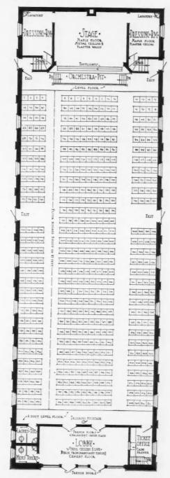
Floor Plan of Theatre Providing 511 Seats. If Constructed for Motion Pictures Only, the Stage and Dressing Rooms Would be Left
