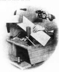
Set at an Angle for Mitre Sawing.
