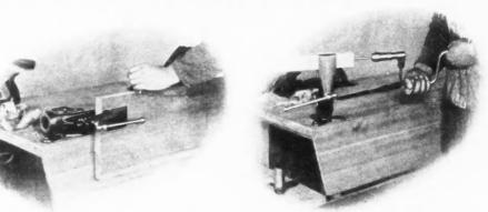
"Carpenter Vise" in Two Positions for Edge Planing and for End Boring.
