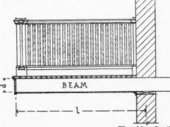
Fig. 4A. Cantilever Beam with a Uniformly Distributed Load.
