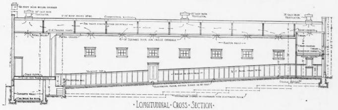
Longitudinal Section Thru Theatre, showing 5-Foot Drop in Floor from the Entrance Doors to the Stage. Operator's Booth for Lantern is Above the Lobby.
