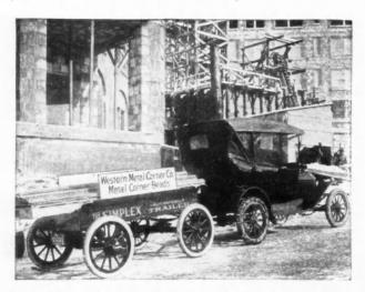
Light Four-Wheel Trailer with Front and Back Wheels Steerable for Short Turns.
