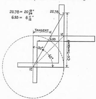
Fig. 1. Illustrating the Tangents for 30 and 60 Degrees.
