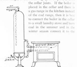
Fig. 4. Hot Water Tank in Kitchen.
