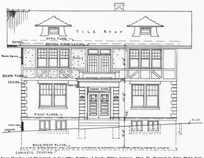
Front Elevation and Photograph of New Office Building of Sparks Milling Company, Alton, Ill., Designed in Swiss Chalet Style, Stone and Cement Plaster Construction, Pfeiffenberger & Son, of Alton, Architects.
