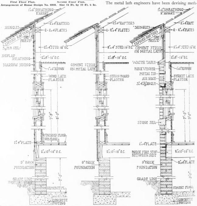
Bevel Siding, Sheathing, Studs, Lath and Plaster.
