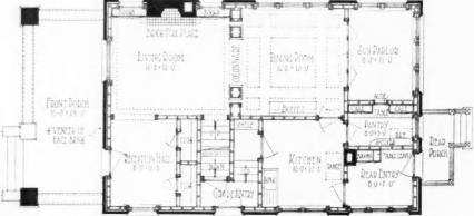
to making the modern rough tex- First Floor Plan of Brick Veneer House. Design No. 6857. Size 26 Ft. by 38 Ft. 10 In.
