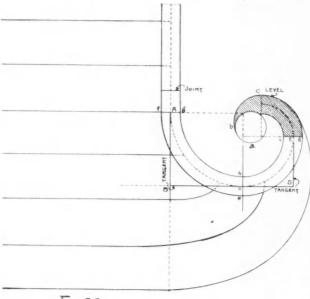
FIG. 32 Plan of the Scroll and Few Steps
