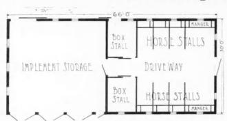
Floor Plan of Combined Horse Barn and Implement Storage, Design No. A380, Illustrated on Page 84. We Can Furnish Complete Set of Blueprinted Working Plans and Typewritten Specifications for only \$6.00.
