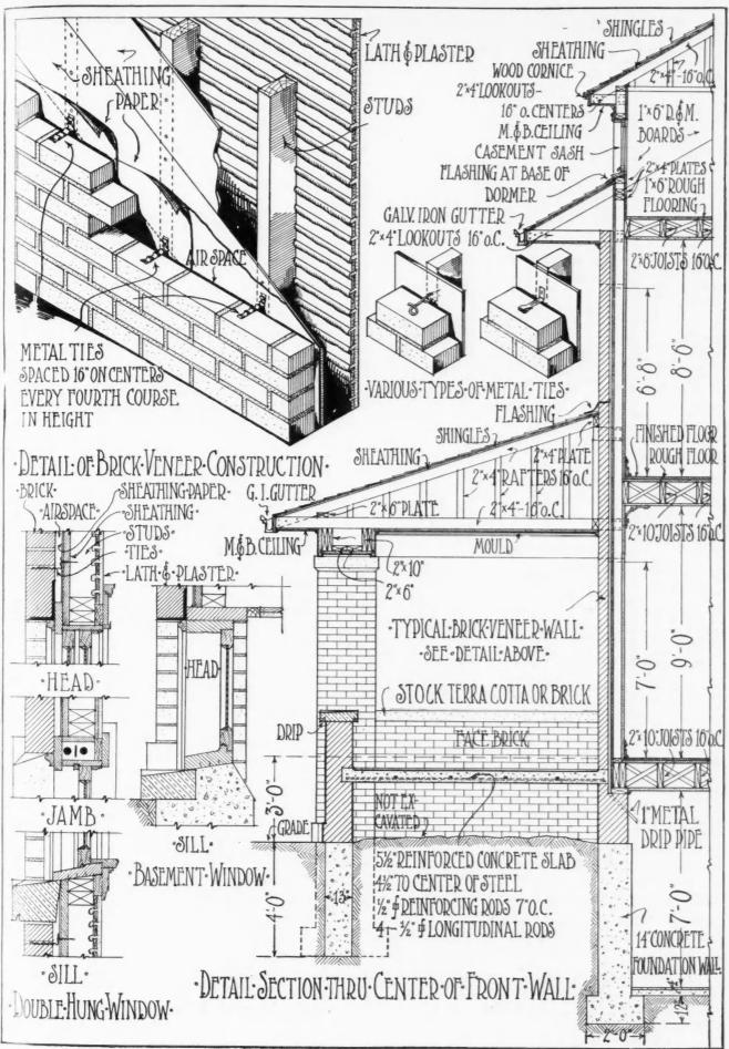
Details of Best Method of Brick Veneer Construction, Calling for Sheathing Boards and Paper Under the Brick—Foundation Provided for Any Soil. For Photograph See Page 59. Design No. 6857.
