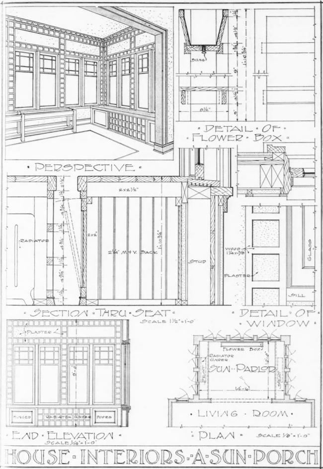
Terspective Sketch, Elevation, Plan and Construction Details of a Sun Parlor Finished in Lattice Style Suggesting the Outdoors.
