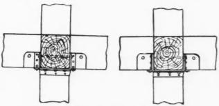
Fig. 10C. A Four-Way Steel Post Cap.
