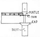
Fig. 10D. Pintle and Post Cap Type of Construction.
