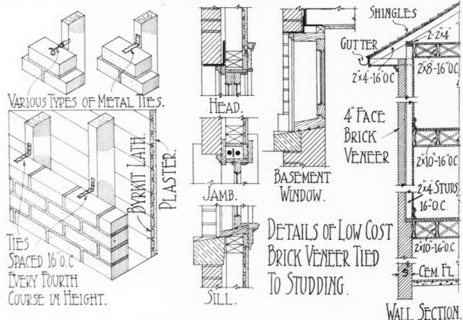
Brick Veneer Walls Constructed in this Manner are Built at the Same Cost as All Frame. For Photograph and Floor Plans See Pages 58 and 59.
