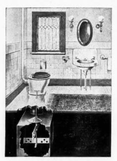
Showing How the United Chemical Closet is Installed.
