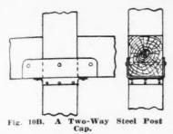
possibly a smaller crushing strength than timber. The plate is also used to obtain an even bearing surface for the wood and to protect it from moisture, likely to be present in concrete or ma-
