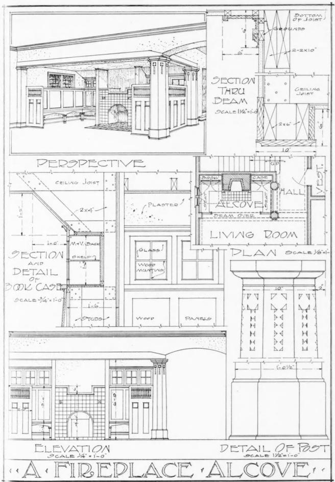
Shetch, Elevation, Plan and Details of Fireplace Alcove Suitable for Large Elaborate Living Room. Designed by Ralph W. Ermeling.
