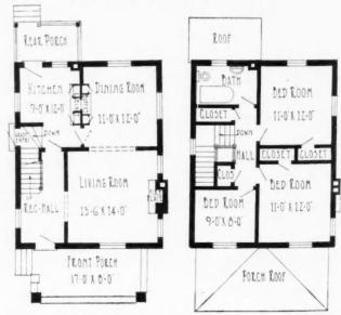
Typical Floor Plan of Six-Room Brick House, Size 22 by 28 Feet.
