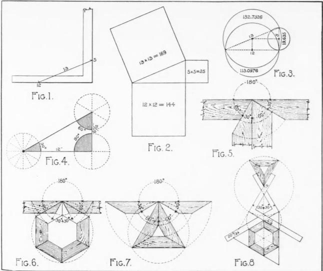
The Steel Square as a Right Angle Triangle for the Solving of All Geometrical Problems.
