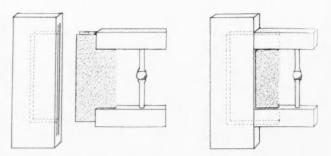
The Metal Braced Joint of the "No Sag" Screen Door.
