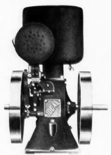
Wheel View of Ideal Engine, Showing arburetor, How Magneto Gears are Direct Exhaust Side of Ideal, Showing onnected, and Spark Plug Just Above Magneto and Large Bearing Boxes. Connected, and Spark Pl Valves on Inside of Hopper
