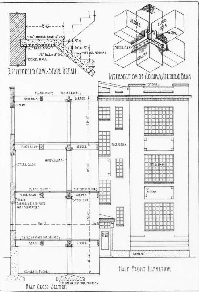
Working Details Standard Mill Construction Factory Building, Design No. 6875, Illustrated on Opposite Page.
