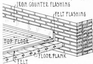
Fig. 11A. Section of Mill Construction Floor Showing Plank, Waterproofing and Wearing Surface,
