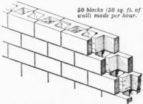
Synstone Double Wall, for heavy construction, 11½" to 18" in thickness, 33½% to 50% hollow. Large saving in cost over brick walls.
