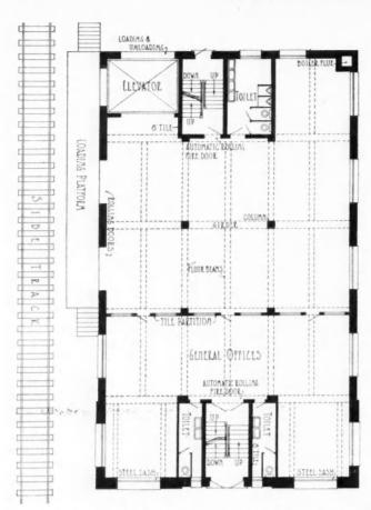
First Floor Plan of Factory, Design No. 6875, Size 48 Feet by 80 Feet. Second and Third Floors Same Without Office Partitions.
