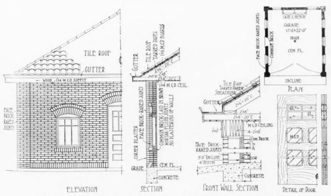
Photograph, Plan, Elevation and Details of Two-Car Brick Garage. Design No. G 174.
