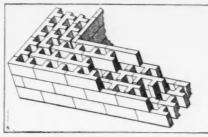
Synstone Wide Wall Construction (multiple air space). 50 blocks (100 sq. ft.) made per hour. Ideal construction for cold storage or packing houses. 194" to as many feet in thickness as desired. Absolutely impervious to heat, cold and moisture.
