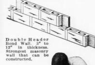
Synstone Machinery is very carefully made and thoroughly complete in every detail, making all these walls and the different shapes and sizes of blocks required for them, by simply changing the cores, which is done in thirty seconds. Operated by common labor, 1, 2 or 3 men. Above estimates (50 blocks, 100 sq. ft. per hour) are based upon 2 men with mixture supplied to them.
