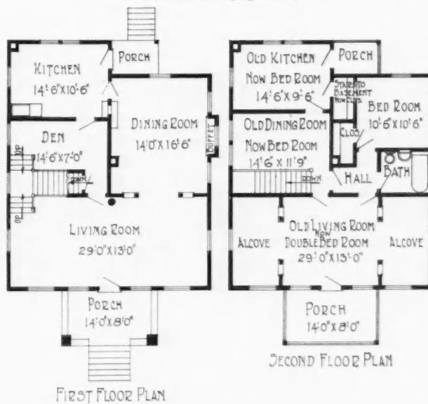
Arrangement of the Remodeled House Showing How the Old First Floor Plan Became the New Second Floor Plan Without a Great Deal of Alteration.
