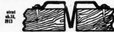
End view showing joint open. Provides for expansion or contraction of the siding so nails will not work loose.
