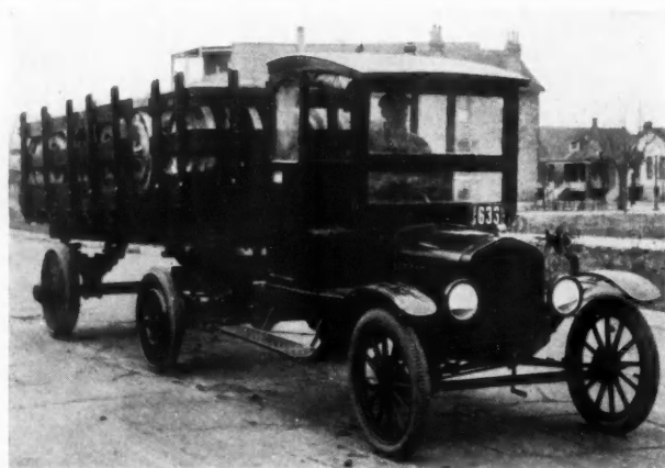
Converted Ford Car with Semi-Trailer Attached by Means of Shock Absorbing Fifth Wheel.
