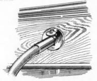
A Considerable Loss of Efficiency A Considerable Loss of Efficiency Is Encountered When One of the Inlets of the Vacuum Cleaning System Is Left Open. To Avoid This Loss, Inlets of the Type Shown Here Are Used. They Close Automatically When the Plug Le With dearer Is Withdrawn.
