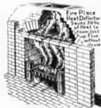
EVERY fireplace should be provided with a heat deflector having a sliding damper operated by knob from face of mantel. Its cost is saved in mason's labor and 50% more heat.
