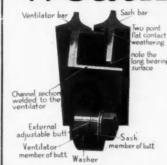
A flat surface, double contact weathering baffles air currents, endeavoring to pass through Fenestra Solid Steel Windows, by turning them at right angles. The cross section of the ventilator to the left shows how this is done. Early makes of steel sash used curved weathering or at best single contact. write for information
