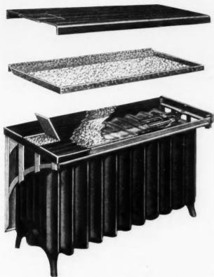
Perspective Detail Showing Parts and Indicating Strength of Humidifler, Which Also Serves as Shelf or Seat.
